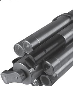
Wiped Conductivity & Temperature sensor in optimal wiping position with o-ring and tie in place.
