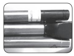
Figure 4 - Sensors installed around the Central Wiper with o-ring in place
