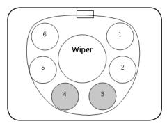
Figure 3 - Optimal Wiped (C/T) Sensor Positions: Ports 3 or 4
