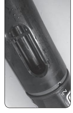
**Figure 10** - Finally, to ensure that the zip tie is out of the way, place the sensor guard back on the sonde.
