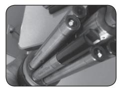
Figure 5 - Wiped C/T sensor in optimal position ready to be secured
