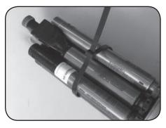
**Figure 7 -** Securing the sensors with the zip-tie with adequate clearance
